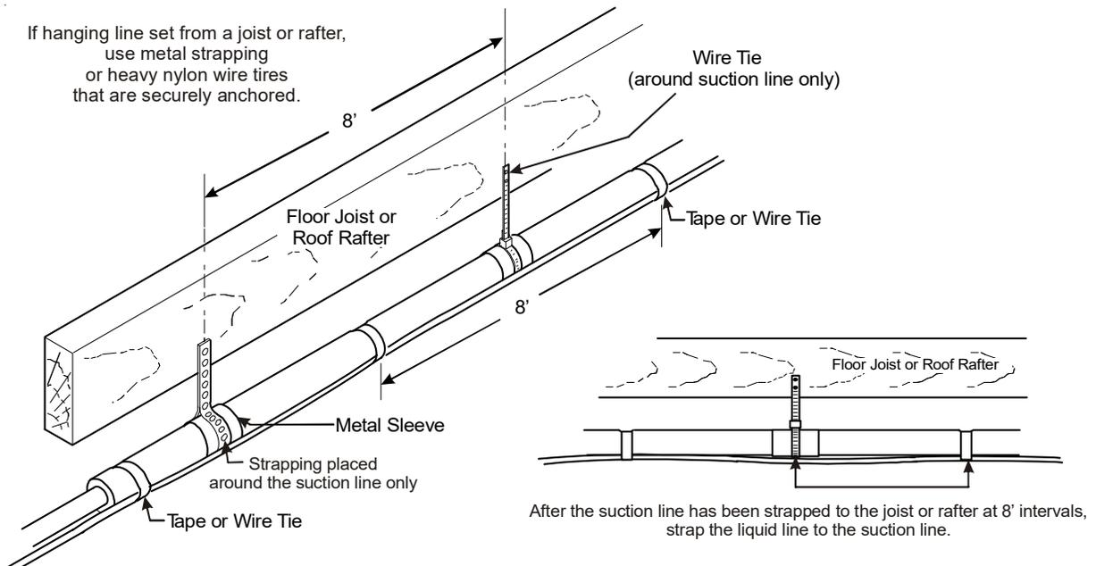
Figure 1-3. Installation of Refrigerant Piping (Horizontal)
