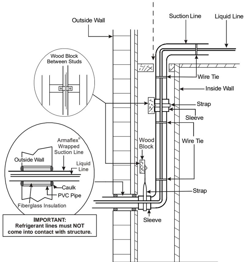
Figure 1-2. Installation of Refrigerant Piping (Vertical)
