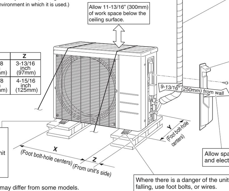
Wrap the insulation pipe with finishing tape from bottom to top.
