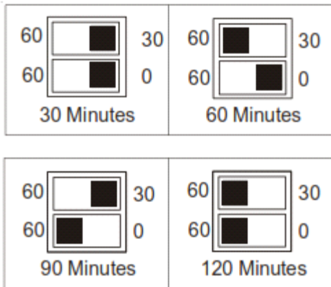
Dipswitch Settings for Selection of Defrost Time
