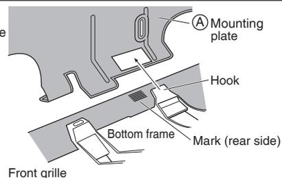
The (A) mounting plate should be installed on a wall which can support the weight of the indoor unit.
