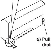
3) Switch around the drain hose and drain plug.
