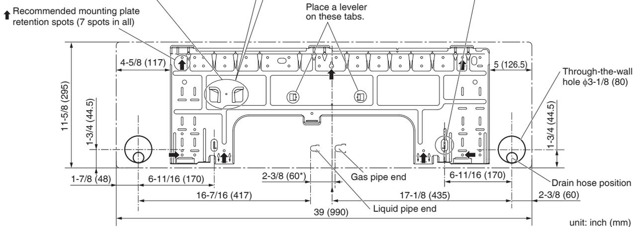
\* Depending on the model, the actual distance between the liquid pipe end and gas pipe end may differ from the distance between those symbols on the mounting plate (the distance listed in this manual). Always measure the actual distance between the liquid pipe end and gas pipe end before installing refrigerant pipes.
