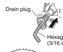
Push the drain plug all the way in using a hexagonal wrench (3/16 inch (4mm)).
