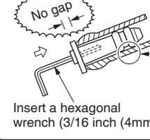
Insert a hexagonal wrench (3/16 inch (4mm)).
