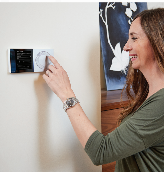
The home screen displays the current temperature, the current system mode, and adjustment slider, as well as icons leading to the top level screens.
