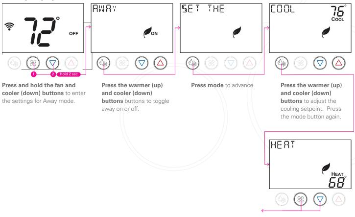
Press the warmer (up) and cooler (down) buttons to adjust the heating setpoint.
