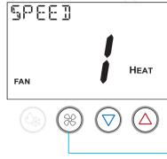
Press the warmer (up) and cooler (down) buttons to cycles through available fan speeds of auto and 1 (low) through 5 (high).
