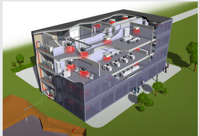
1 Cooling Tower or Dry Cooler 2 Boiler 3 Indoor Units 4 Refrigerant Pipes 5 Condensing Units 6 Water Loop Piping
