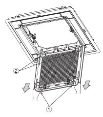
① Pull the air filter end inclined downward and unhook the hooking hole of the air filter from the grille projection. (both right and left)
