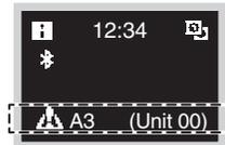
Press and hold
