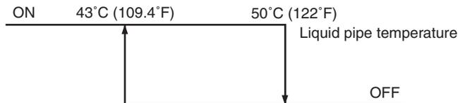
2. The heater control (ON/OFF) is conducted by converting the heater temperature into the condensing pressure equivalent saturated temperature (Tc) according to the temperature detection through the high pressure sensor (S1NPH) of the outdoor unit.
