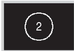
When the U5 error code appears, press
